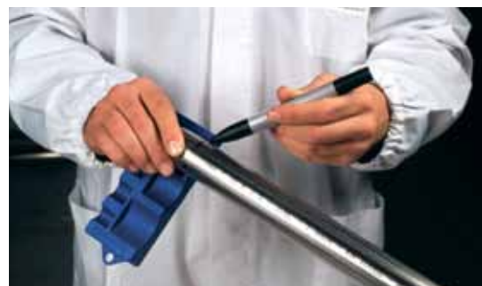
Figure 28 - Marking the insertion depth
