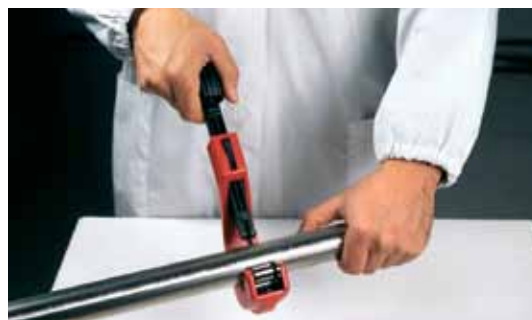
Figure 25 - Cutting the pipe to length
