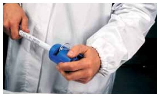
Figure 29 - Stripping (Steelpres PP coated)
