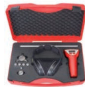
Acoustic leak detection of heating installations
