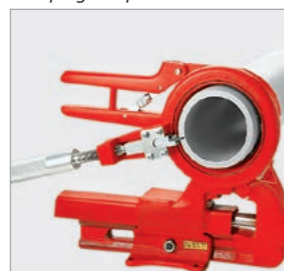
Clamping in a parallel vice
