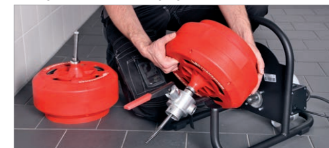
Interchangeable drum for different working ranges
