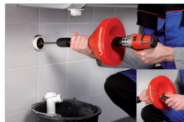
Electrical operation with cordless drill
