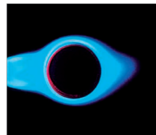
High flame temperature based on cyclone swirl
