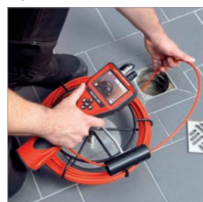
Inspection of floor drains
