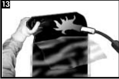
Partially remove the release liner from the sleeve (~15 cm from the edge) and gently heat the adhesive along the underlap with a torch.
