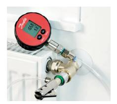
To ensure maximum energy savings the renovated heating system was commissioned with using the dP tool™. This simple tool measures the available differential pressure directly in the *Dynamic Valve*™. The pump pressure of the Grundfos MAGNA was lowered while the required differential pressure in the furthest located valve stayed intact.
