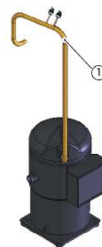
Fig. 4: The pressure pipe (1) should get hot during operation
